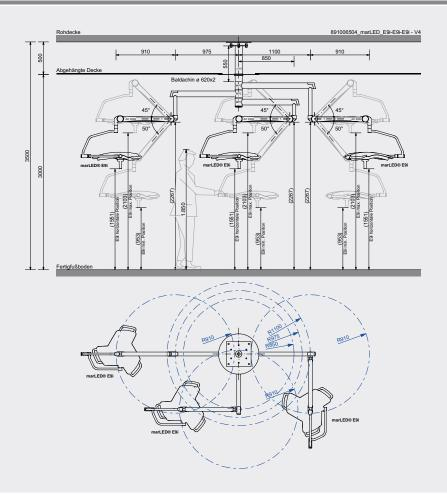
89-100-65-04  $\label{eq:constraint} {\rm marLED}^{\circledast} \mbox{ OPL-Kombination E9i/E9i/E9i} - {\rm deckenmontiert, Standard}$
