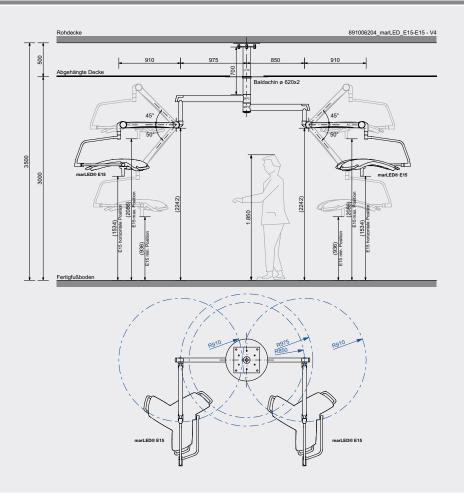
89-100-62-04  $\label{eq:constraint} \mbox{marLED} \mbox{$^{\circledcirc}$ OPL-Kombination E15/E15} - \mbox{deckenmontiert, Standard}$
