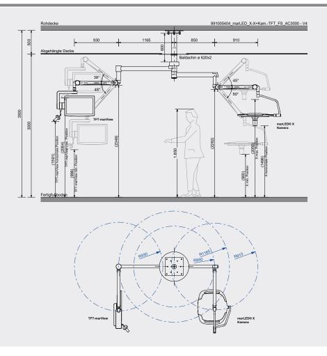
89-100-52-04  $\mbox{marLED} \mbox{\ensuremath{\$}} \mbox{ OPL-Kombination X+Kamera/marView AC3000} - \mbox{deckenmontiert, Standard}$
